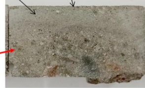
Cores ~83 mm diameter
