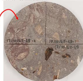
Cores ~83 mm diameter
